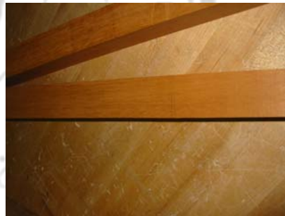
Jim Stevens and Tony Albano brought in the legs and described how they tapered the legs on a planer table
