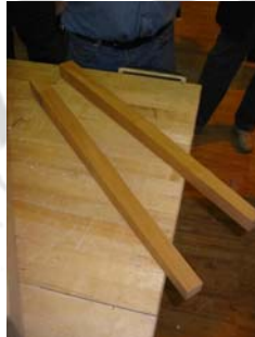
Jim Stevens and Tony Albano brought in the legs and described how they tapered the legs on a planer table
